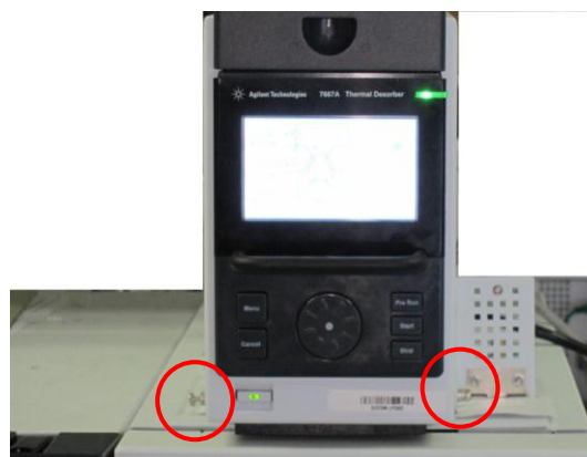
Figure 22 Fixed screws on the Mini TD
