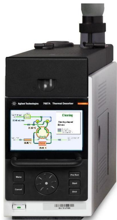
Figure 1 Front View of the Entry version Mini Thermal Desorber (G4370A)
